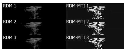
Figure 5 Example of XENSIV RADAR data visualization for the MultiMedaLIS Dataset. From left to right: Range-Doppler maps captured by three separate receiving antennas, followed by an MTI (Moving Target Indication) map highlighting motion-based targets.
